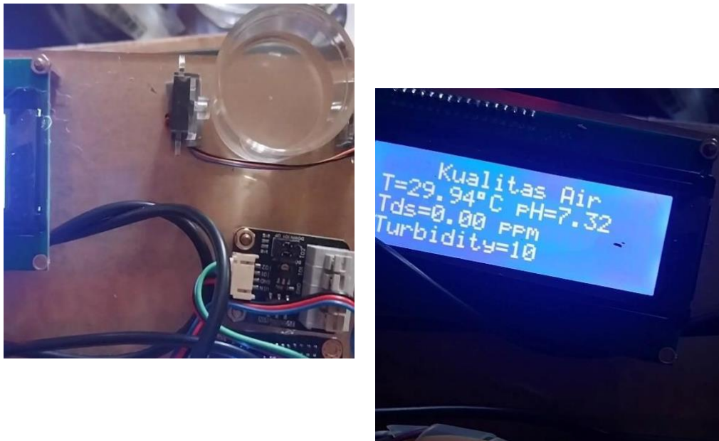
Figure 22. Clean water testing
