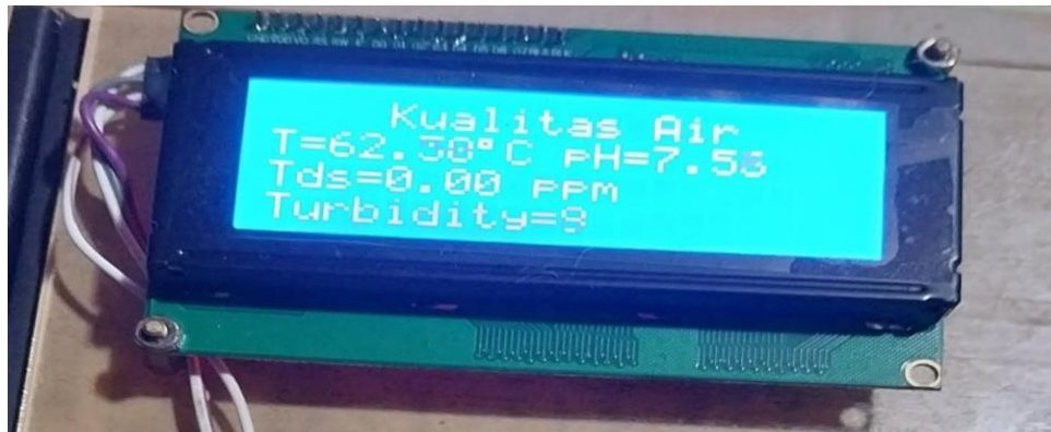
Figure 26. Temperature Sensor Display Monitor Screen
